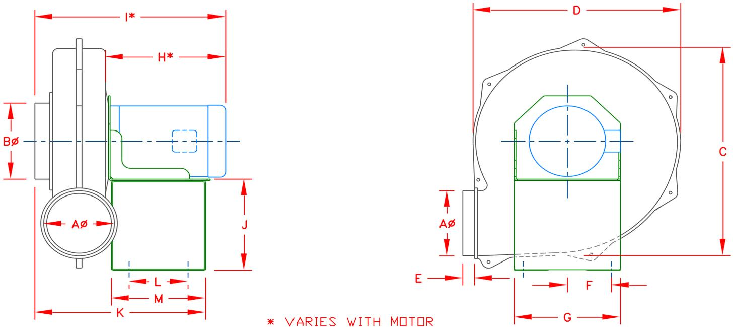
The Motor Frame is normally decided by the factory based on H.P. and the RPM of the fan. The 56 frame is normally used on up to 1 H.P. motors, and 143T is used up to 3 H.P. in most cases. If you require a specific frame for your selected motor, contact your dealer as some fans can interchange between motor frames for special needs.
