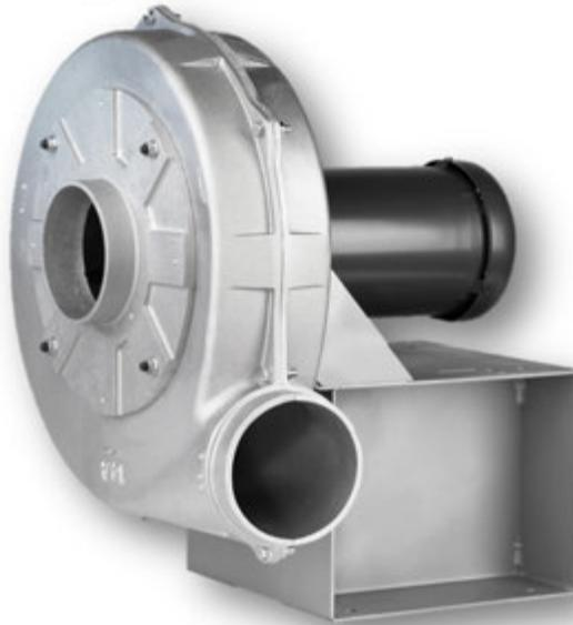
This exhaust fan is designed for the purpose of exhausting most particulates as well as volatile organic compounds (VOC's) created by internal combustion engines. These fans feature high pressure 3/16" minimum thickness radial flat wheels, direct drive, and are AMCA Type B spark resistant. Housing shall be of Aluminum/Magnesium alloy created by 2-piece construction with gaskets and steel hardware. Fan shall be tested and be in accordance with AMCA Standard 210.
