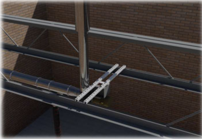
Ceiling Joist Mounting- Unistrut Hung from Ceiling Joists
