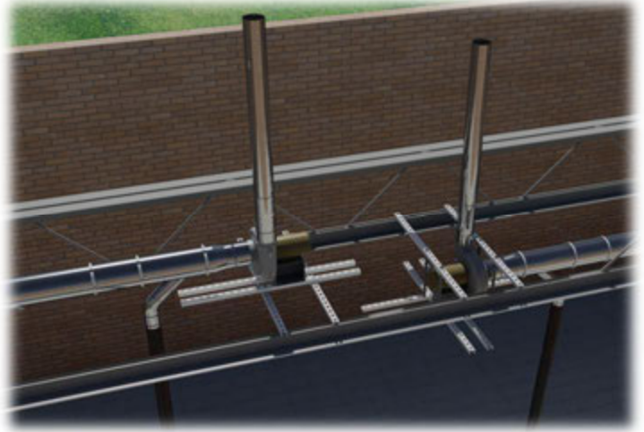
Unistrut Structure- Unistrut can be Fabricated into Joists via Hardware
