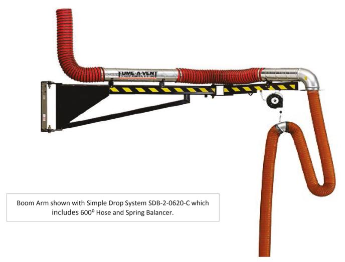
**Shown:** Pivoting Articulating boom arm simple drop system, with a balancer for hose storage. This system works great for shops with overhead cranes or high ceilings that prevent the user of other overhead systems. The system stores tightly against the wall when not in use, and swings out over or between bays when needed. The Articulating arm is able to scissor at its midpoint for maximum flexibility.
