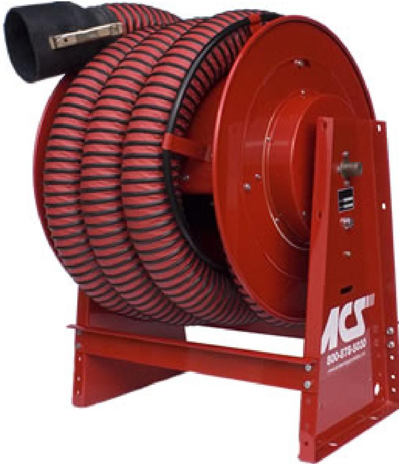
Shown above: **Fume-A-Vent** Model HRS-LD Spring Hose Reel with 4" x 25' Series 3 400° rubber impregnated polyester hose. Optional TPA-03-0404 tailpipe adapter with spring clamp.
